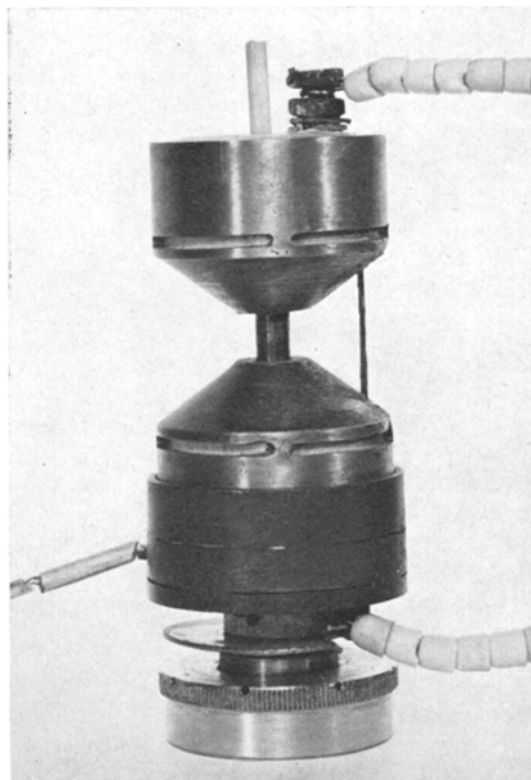
Figure 2 Single-crystal heater for use on a diffractometer.
